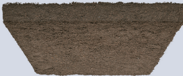
FD Soil Artificial soil with specific gravity reduced to about half of natural soil
